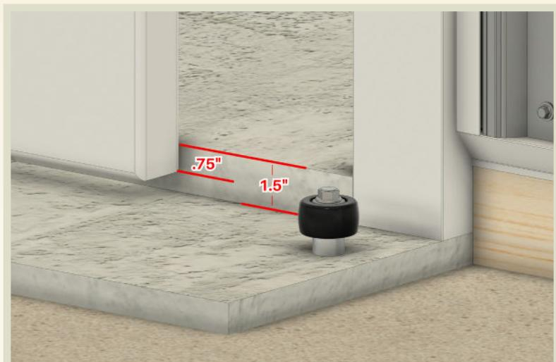
Concrete Apron with Step for Weatherproof Seal
