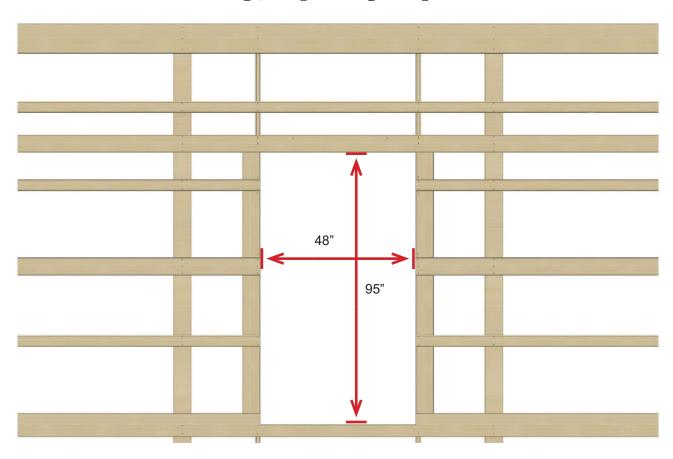
Image shows suggested framing for pole barn installation. Recommended rough opening size is 48" x 95".
