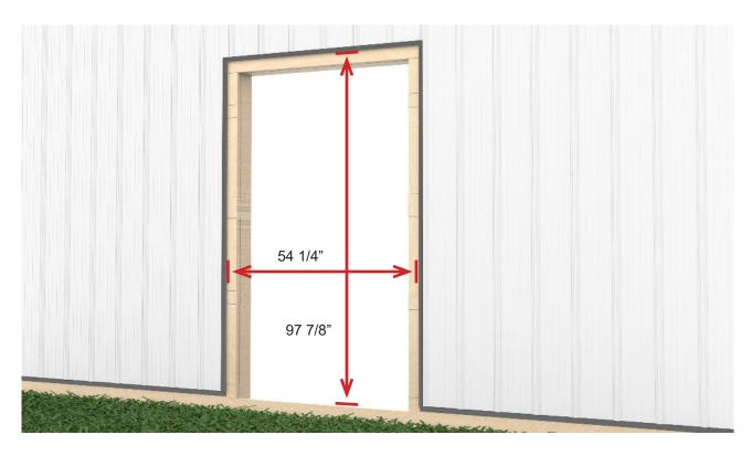
Although not recommended by J&E, siding can be installed before the door. Allow 1/16" gap on sides and top. Refer to print for outer door dimensions.
