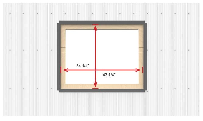
Although not recommended by J&E, siding can be installed before the window. Allow 1/16" gap on sides and top. Refer to print for outer window dimensions.
