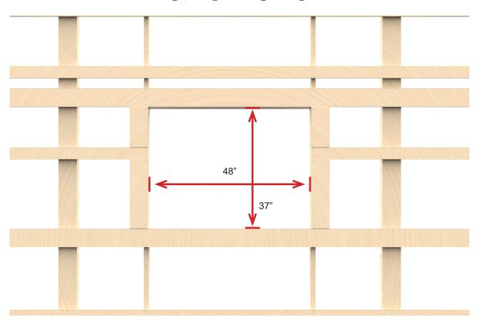
Image shows suggested framing for pole barn installation. Recommended rough opening size is 48" x 37".
