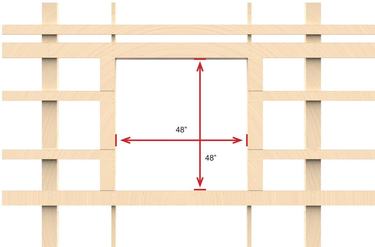
Image shows suggested framing for pole barn installation. Recommended rough opening size is 48" x 48".
