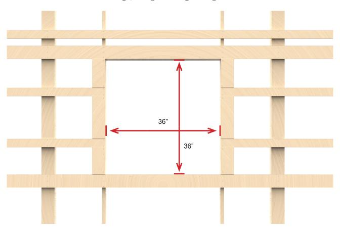
Image shows suggested framing for pole barn installation. Recommended rough opening size is 36" x 36".
