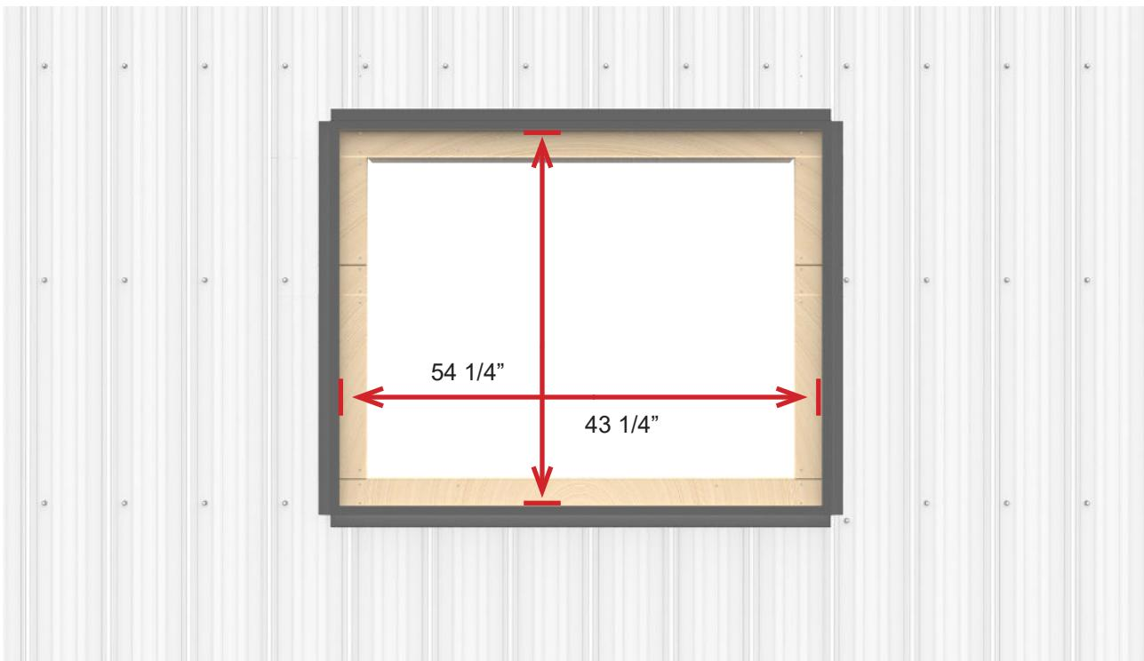
Although not recommended by J&E, siding can be installed before the window. Allow 1/16" gap on sides and top. Refer to print for outer window dimensions.
